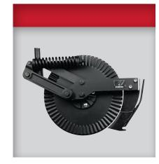
Designed for no-till planting conditions, this 17 in. (432 mm) disc and knife work well in firm, no-till soil that has residue on the soil surface. The disc cuts residue at the soil surface, and the trailing knife places the fertilizer with minimum soil disturbance.
