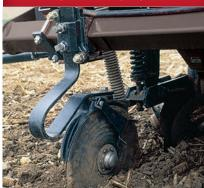
Designed for conventional and minimum-till applications. Two 13.5 in. (343 mm) diameter discs are C-spring mounted to an adjustable clamp.
