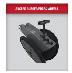
Improve seed-to-soil contact in heavier soil and moderate no-till conditions. Adjust wheels by offsetting them or changing width from 1.25 to 2.88 in. (32 to 73 mm) for improved performance at various seed depth and soil conditions. Adjustable down pressure: 50 to 133 lbs. (23-133 kg.).
