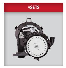
vSet2 with vDrive provides perfect singulation. By using a flat disk, it doesn't have a cell with a "preference" for a certain seed size. The flat disk, combined with a singulator riding on the edge of the disk knocking off extra seeds, gives you 99% singulation accuracy in corn and soybeans without adjustments to vacuum, disk or singulator.
