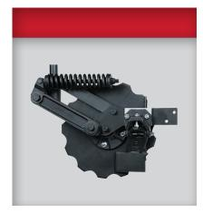
Designed for no-till and minimum-till applications, this single-disc fertilizer opener features an austempered side profile knife to place fertilizer up to 4 in. (102 mm) deep, providing effective placement of fertilizer with minimal adjustment.
