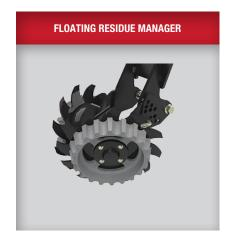
13 in. (330 mm) SharkTooth or finger wheels and depth bands provide aggressive residue movement from the path of the row unit. The unit-mounted residue wheels float over the surface, and the depth bands assure the right depth of operation.
