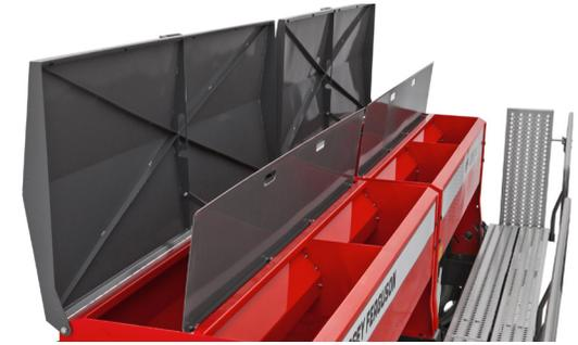
A moveable partition allows easy adjustment of the seed/fertilizer ratios – particularly useful when planting soybeans.
